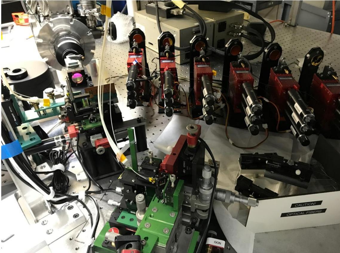
*Fig.5: C-RED One mounted on the MIRC-X imager
